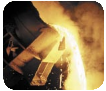
Tapping from ASM Converter in Progress
