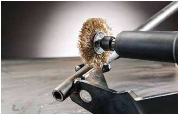
Welded seam machining using a circular brush with shaft and twist-knotted wire bristles.
