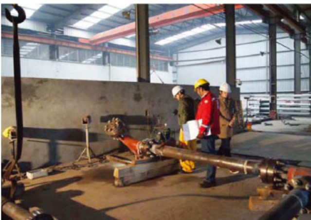
Inspection after hydrostatic test
