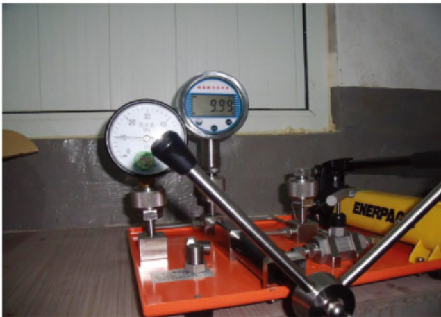
Check pressure gauges before Testing
