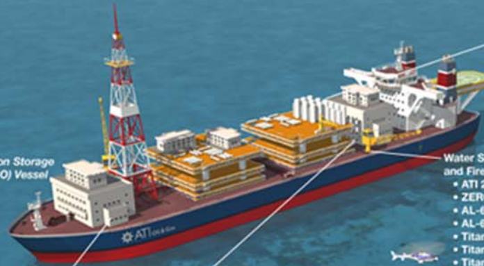
Instrumentation Tubing, Piping & Pipe Racks • ATI 2003 ® Lean Duplex • ATI 2205 ™ Duplex • ATI 316L Stainless
