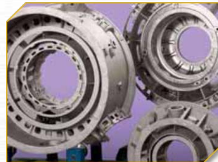
Castings - Titanium Investment, Titanium & Zirconium Rammed Graphite, & Iron
